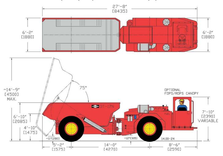
The DUX MODEL DT-17N, 17 metric tonne payload capacity high-speed articulated four-wheel drive haulage truck is only 1.9 meters wide. Designed to operate in confined areas, small drifts and tunnel projects, the ruggedly built DT-17N offers high capacity production hauling of ore, waste and backfill on the level and on steep ramps. Long trouble-free service and a low operating cost-per-tonne are guaranteed on all types of development projects with the DUX DT-17N.
